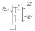
Note: If side jamb has a wide groove which prevents the clip from being fastened flat against the jamb, place the supplied wood shim behind the clip before fastening to keep it level.
